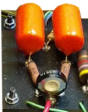
Trim tab inside a boutique amplifier to tune the circuit to a custom level.
